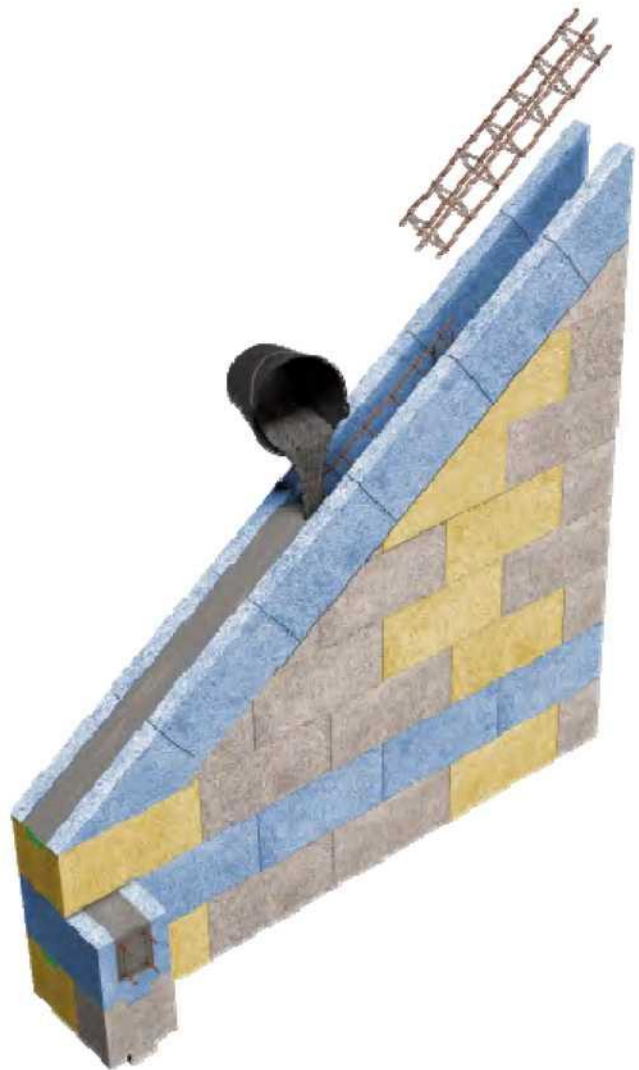
Figure 39: casting the gable linkage concrete
