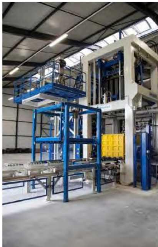
Figure 21: Side view of the block press from the hemp concrete exit side
