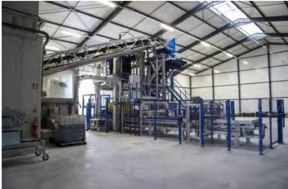
Figure 20: Side view of the block press from the hemp concrete arrival side
