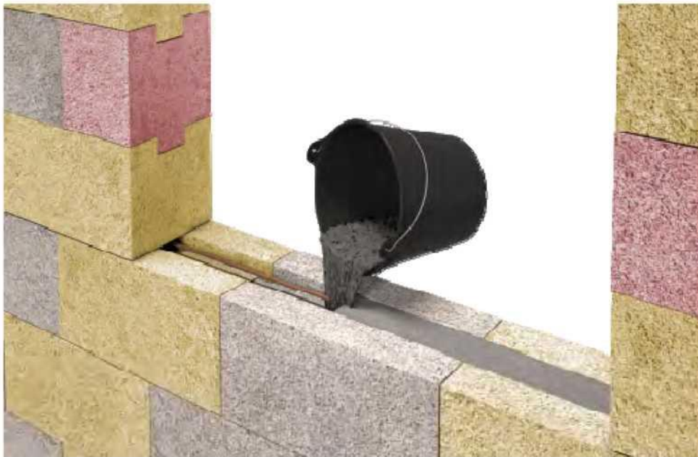
Figure 43: casting window reinforcement concrete
